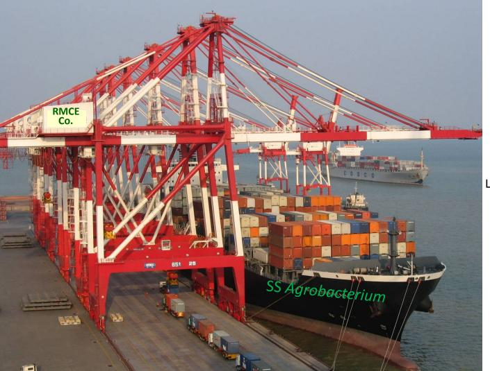
Shown is a gantry crane loading a large amount of cargo onto a container ship
